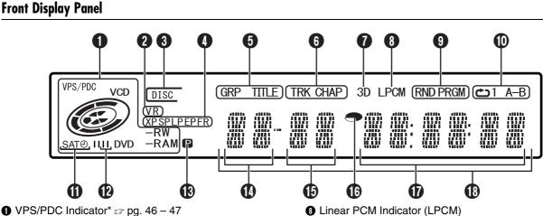
Appears when checking if the station being received transmits a VPS/PDC signal.
